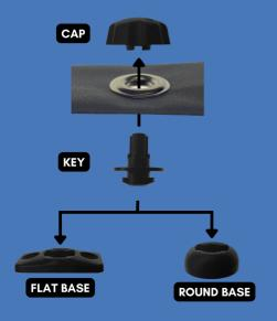
The Cap and Key are designed to be permanently installed through a 9.5–10mm (3/8") eyelet or grommet with a finished thickness of <5mm. This allows the parts to rotate freely.
