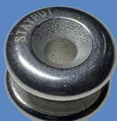
The New Stayput® Stainless Steel Shock Cord Knob provides a premium look with its polished finish and low 11mm profile. It suits up to a 6mm shock cord and is secured using an 8g countersink screw or suitable rivet.
