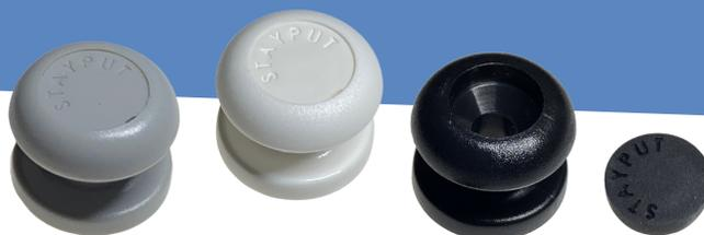
The **Stayput® Shock Cord Knob with Cap** is our premium nylon Shock Cord Knob. It is the same size as our Standard Stayput® Shock Cord Knob but we have deepened the countersink and added a neatly fitting cap to cover the screw or rivet. The result is an attractive finish with concealed fixing. It has been designed to suit a 3/16" / 4.8mm rivet or 8g countersink screw.
